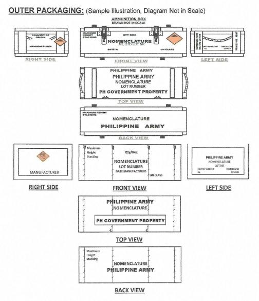
**Note:** The illustrated diagram is just an example purposely to serve as reference. Placement, font size, and font style are manufacturer's standard. Refer to Technical Specification for the minimum required markings.
