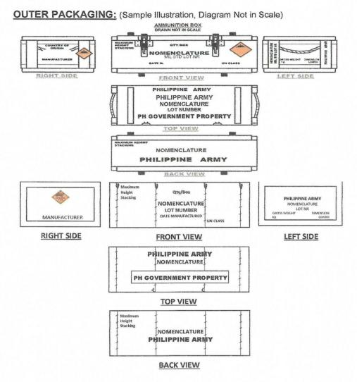
**Note:** The illustrated diagram is just an example purposely to serve as reference. Placement, font size, and font style are manufacturer's standard. Refer to Technical Specification for the minimum required markings.
