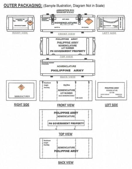
**Note:** The illustrated diagram is just an example purposely to serve as reference. Placement, font size, and font-style are manufacturer's standard. Refer to Technical Specification for the minimum required markings.
